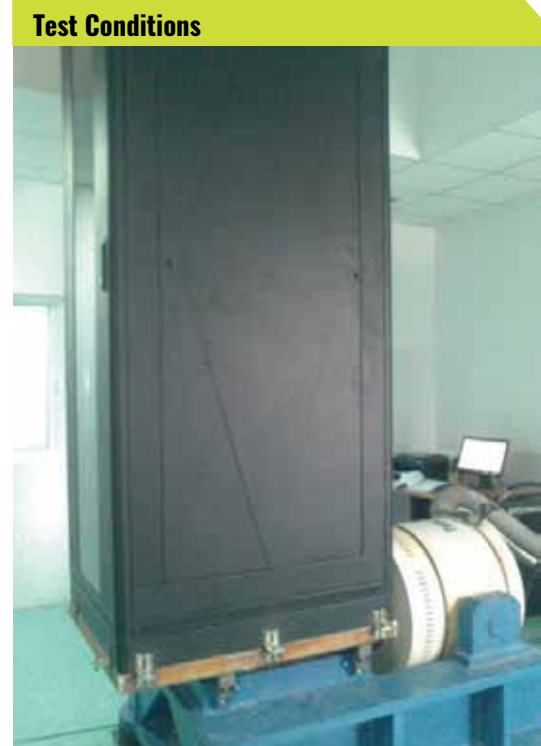
Dynamic load, vibration and mechanical impact tests (DL4)
